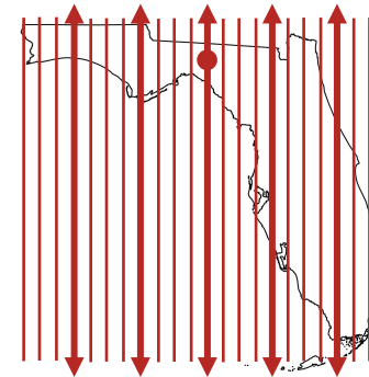
RANGE LINES Vertical lines 6 miles apart
